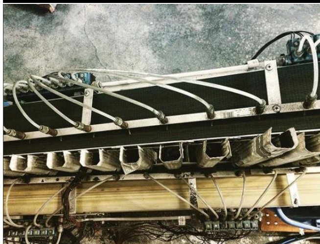
Bird's eye view of Numan sorting machine. Coins ride on the conveyor belt at the bottom of the photo and are pushed into sorting bins
